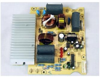
KW712921 - INDUCTION COIL AND NTC ASSEMBLY
